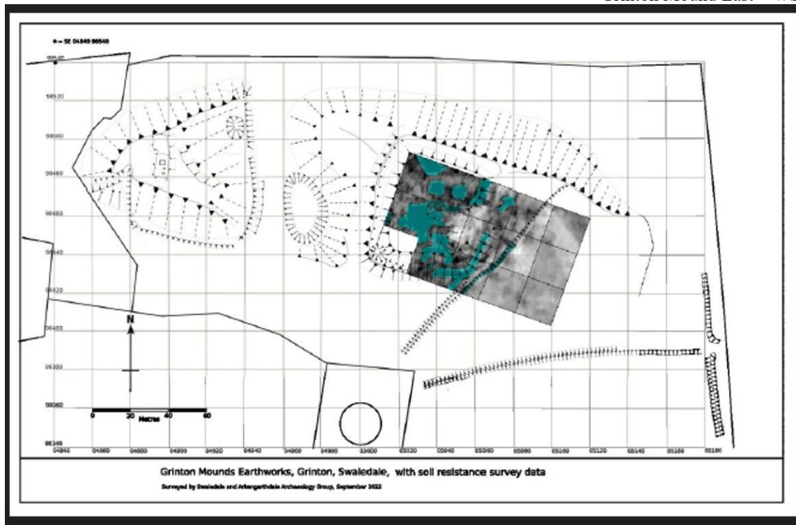
Plate 6 : Resistivity survey data with features highlighted; surveyed SWAAG 2022 NB: the blue probably indicates a stone/sand surface
